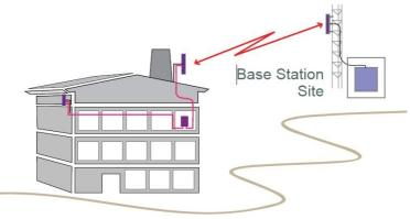
The D-CSR 3604 can also be used to provide coverage in shorter tunnels. Longer tunnels can be covered by connecting the repeater to an OMU (Optical Master Unit) that feeds a number of fibre fed repeaters.
