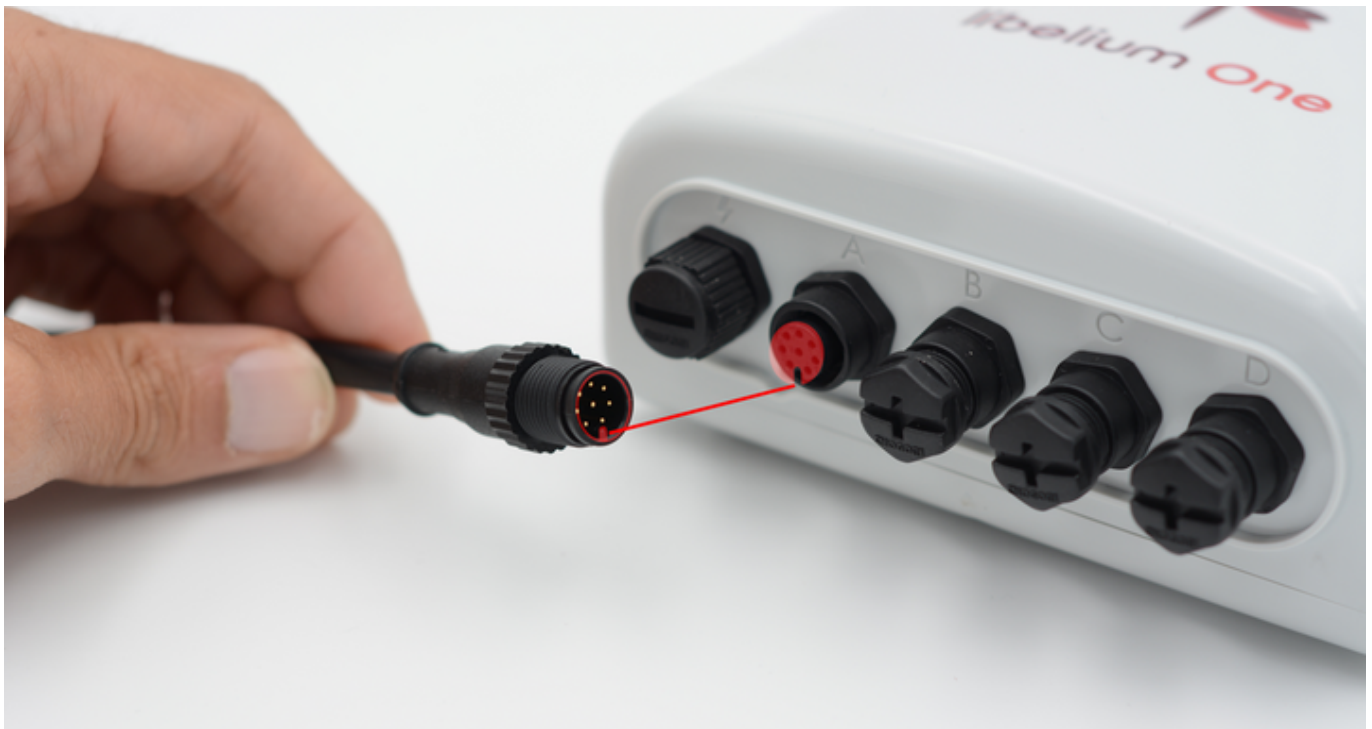
Align the connector before trying to connect the sensor
