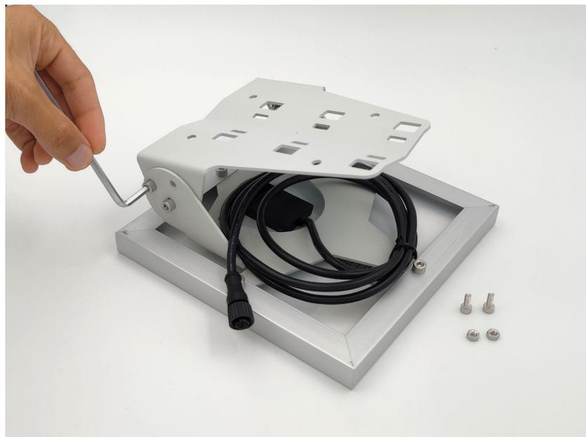
Assembling the screw in the working position
