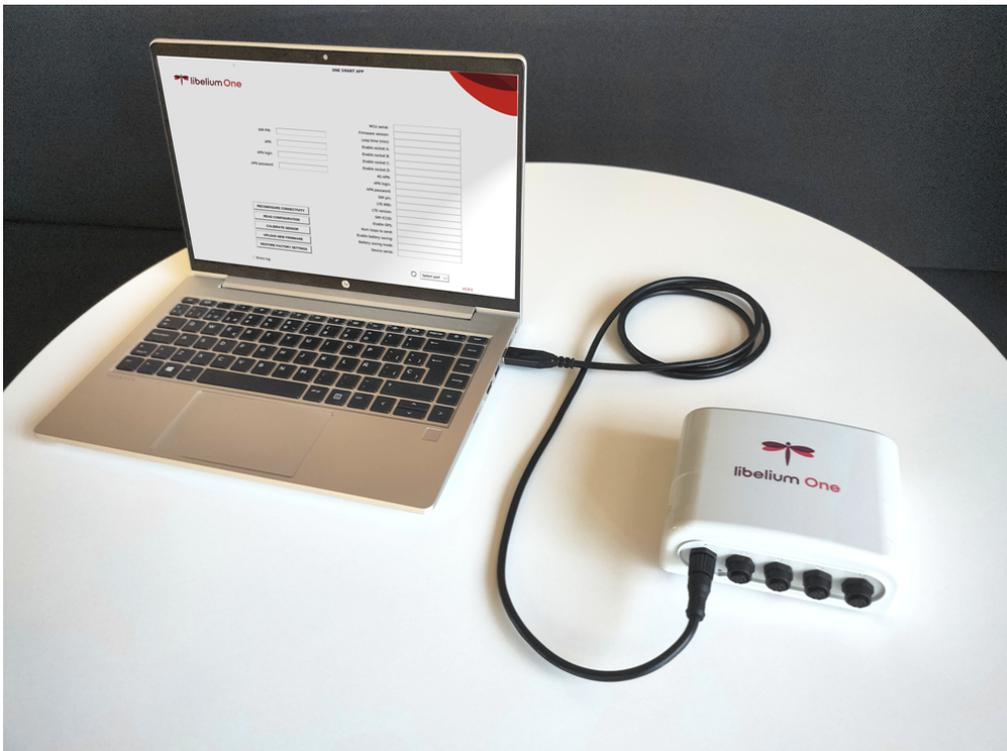
Libelium One node connected to a laptop using the One programmer accessory
