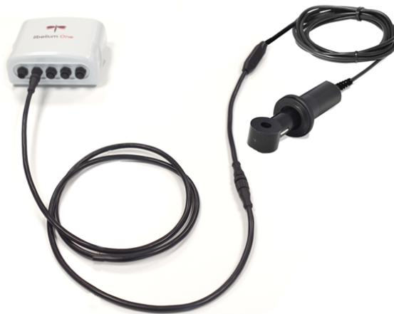
One node with an extension cord in series with the sensor
