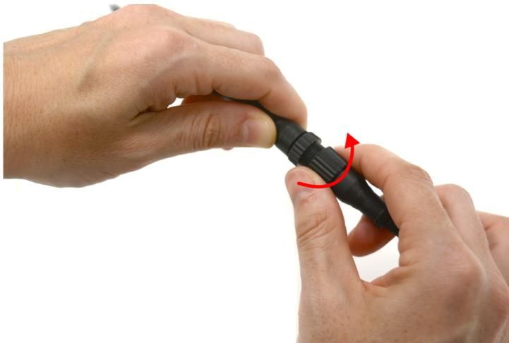
Connecting an extension cord in series with the One sensor
