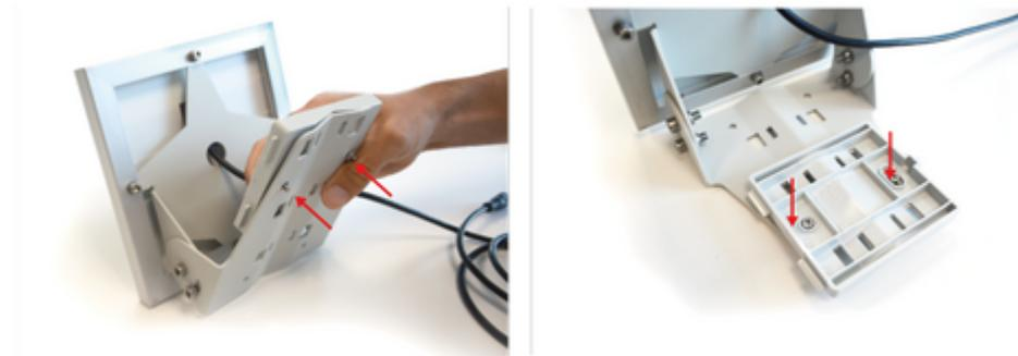
Mounting the solar panel with the node
