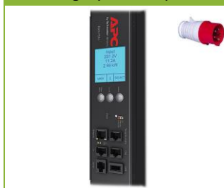
Rack PDU 2G, Switched, ZeroU 16A, 400V, (21)C13 & (3)C19 Cord Length (1.8 meters) IEC309
