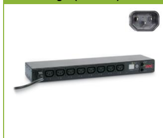
Rack PDU, Switched, 1U, 10A 230V, (8)C13 Cord Length (2 meters) IEC320
